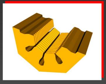
Unique, extreme high-power, highly overmoded, HOM damped, switchable structure.
