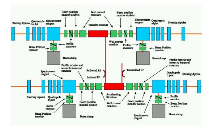
1. Power Extraction Structures (PETS) in what is called the Transfer Structure
