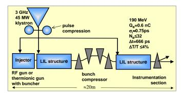
A zero<sup>th</sup> order design based on the reuse of LIL structures is shown in the figure above. The front end can be either a thermionic injector or a RF gun photo-injector. Appropriate instrumentation for beam energy, emittance, current and time structure is mandatory.
